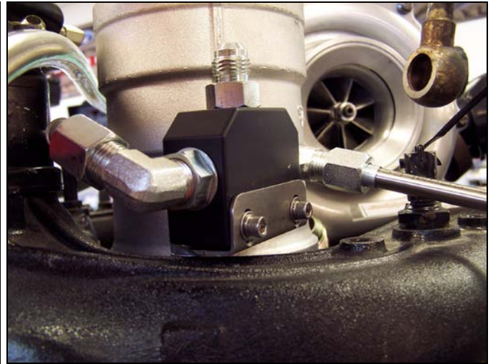
Bowl Delete Block Installed & Tube Connected
