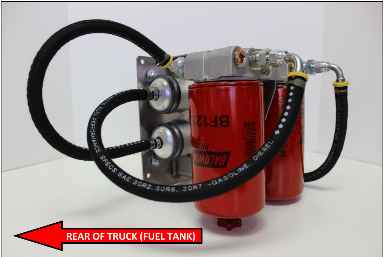
View from PUMP INLET (Fuel Tank) Side – Use this Picture for Hose Routing
