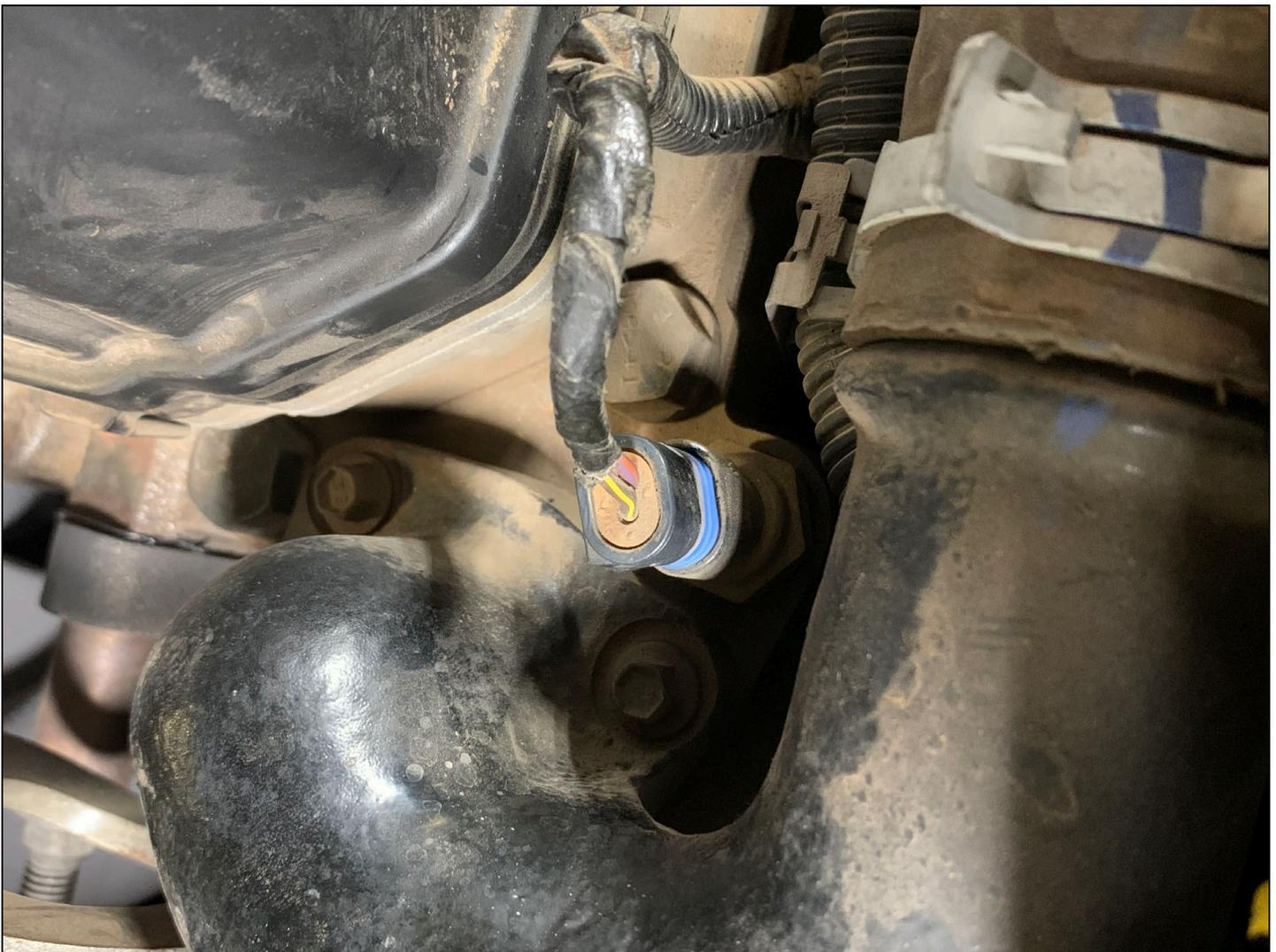
FIGURE 1 – COOLANT TEMPERATURE SENSOR
