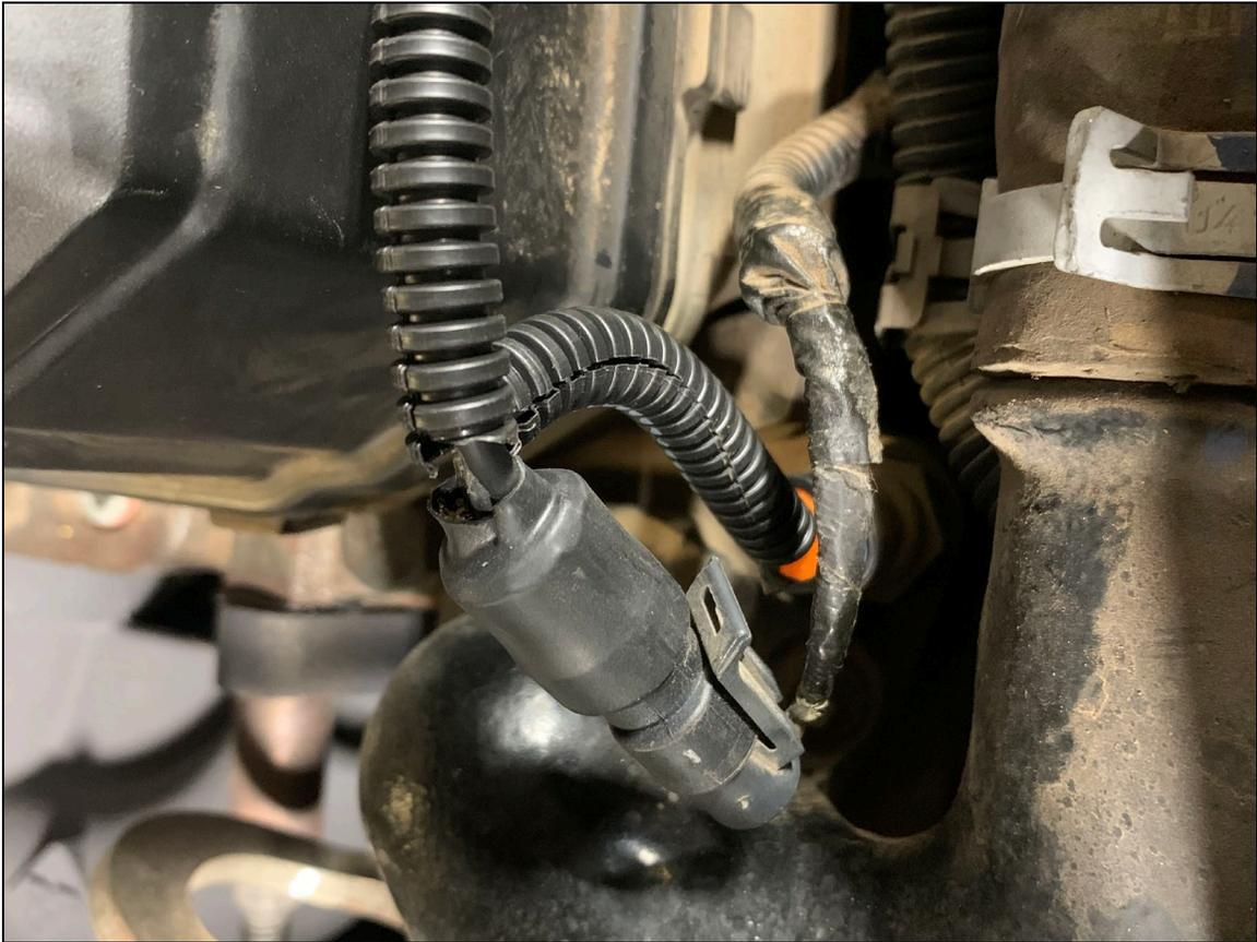
FIGURE 2 – FAN CLUTCH ACCELERATOR INSTALLED
