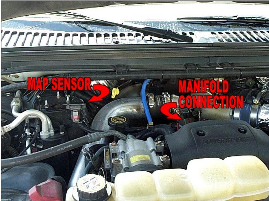
Figure 1 – Location of MAP Sensor and Manifold Connection
