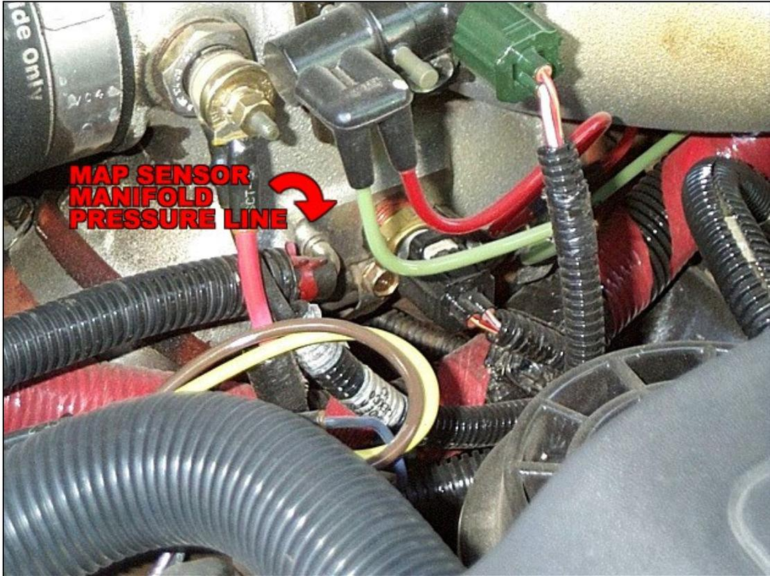
Figure 3 – Location of Manifold Pressure Line
