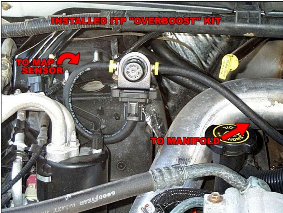
Figure 4 – Driven Diesel "Overboost Annihilator" Kit Installed
