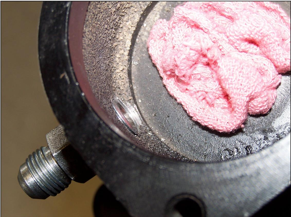
Figure 6 – Fitting Installed Flush with Inside Surface
