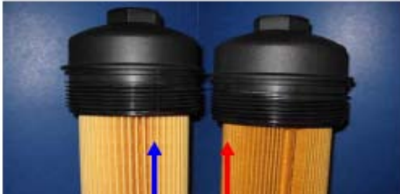
Figure 5 Competitor "A" element body is .250" shorter than the Motorcraft element allowing element to float in housing
