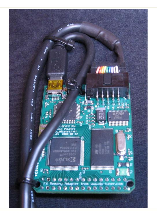
Install the switch and USB cable on the chip. Secure the wires with the supplied zip ties.
