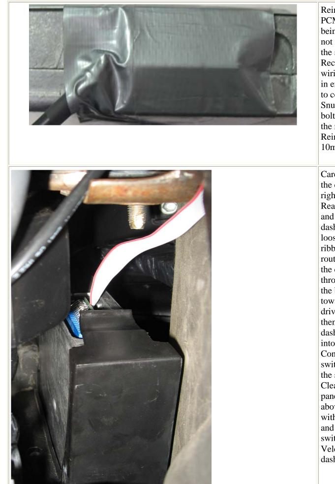
Reinstall the PCM in tray, being careful not to pull on the switch wire. Reconnect wiring harness in engine well to computer. Snug the 10mm bolt. Reinstall the rubber seal. Reinstall the 2 10mm nuts.
