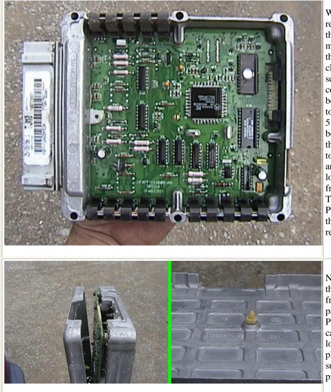
With the PCM removed from the vehicle, you may now begin the process of cleaning the service connector. The best method is to remove the 5.5mm (7/32") bolts that hold the PCM together. There are 6 of them located on the front cover. This is how the PCM looks with the cover removed.
