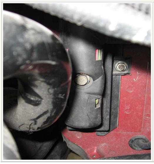
In the engine compartment, there is a wiring harness connected to the PCM. Remove the 10mm bolt in the center of the harness, and pull away from the PCM. Remove the 2 10mm nuts holding the rubber seal and remove the seal. Pull the PCM out into the engine compartment.
